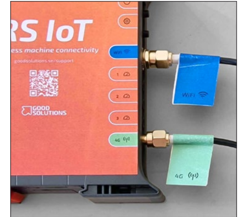
Connect the antenna to the SMA-contacts on the side of RS IoT.
